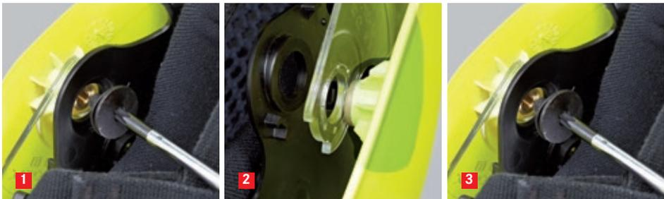
First unscrew the (hexagon socket) screws on both sides (see Fig. 1). Then pull the visor out of its mounting (see Fig. 2).
